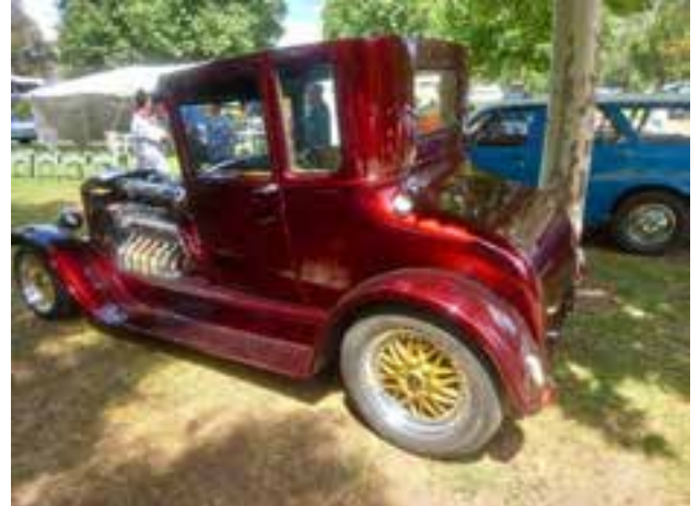
Something unexpected, again using modern chassis, body and other components, was this "Tophat" Model T Ford with a V12 Mercedes motor and drivetrain!
