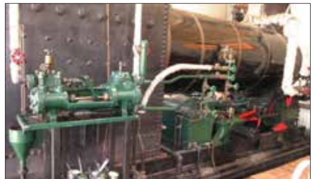
1880s steam engine, restored and fully functional, still runs the generators on these special occasions.
