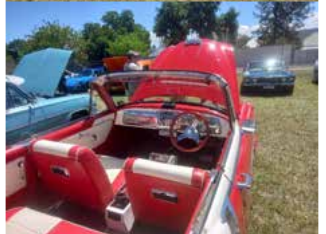
An FC Holden convertible conversion, apparently done many decades ago. The overall effect was excellent, with the doors lengthened four inches to allow easy access to the rear seat. The two-tone paintwork and upholstery added to the
